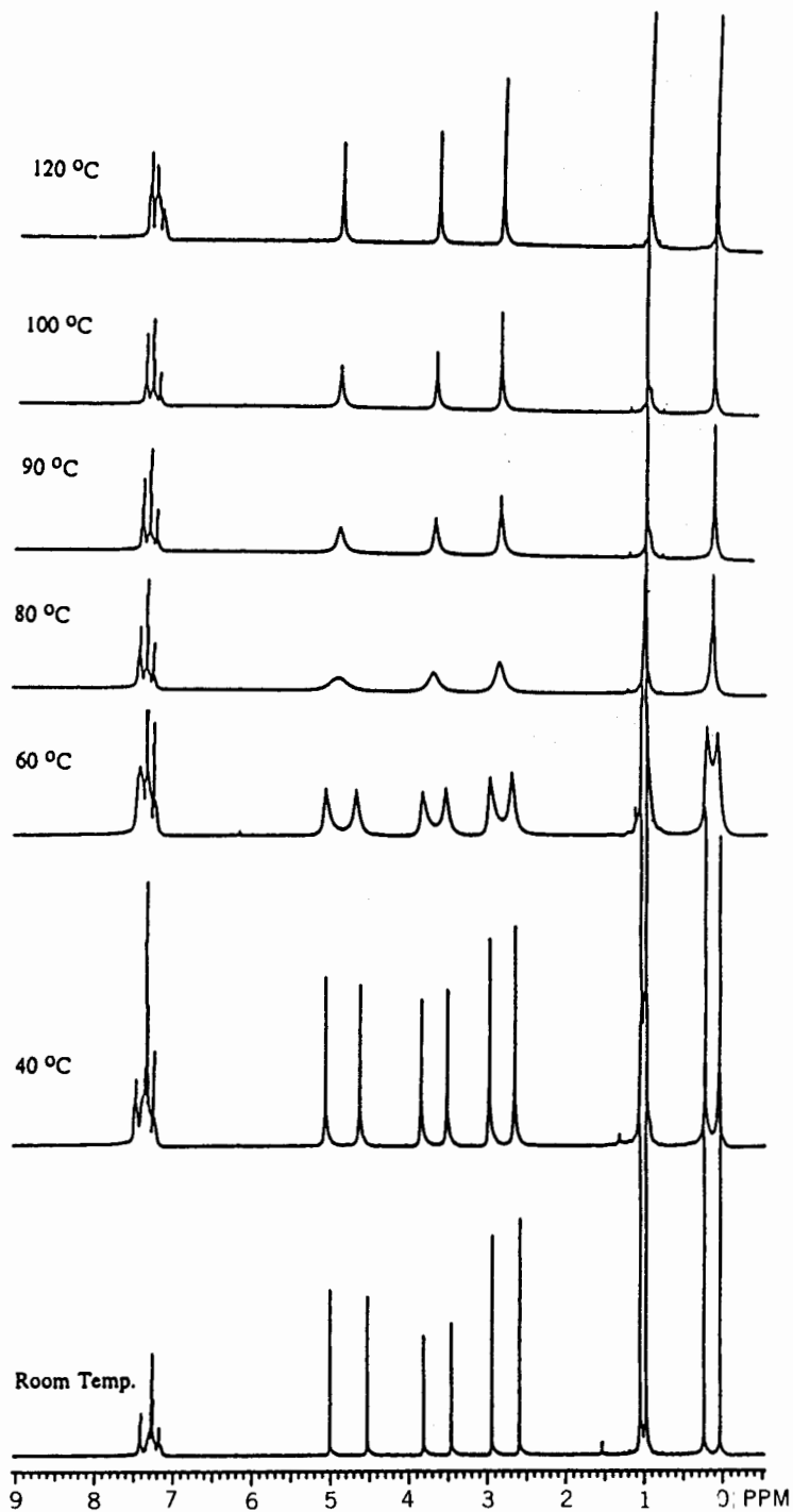
Figure 10.8. The 500-MHz ^1\text{H} spectrum of compound 10-15 (review problem 10.1) as a function of temperature.
