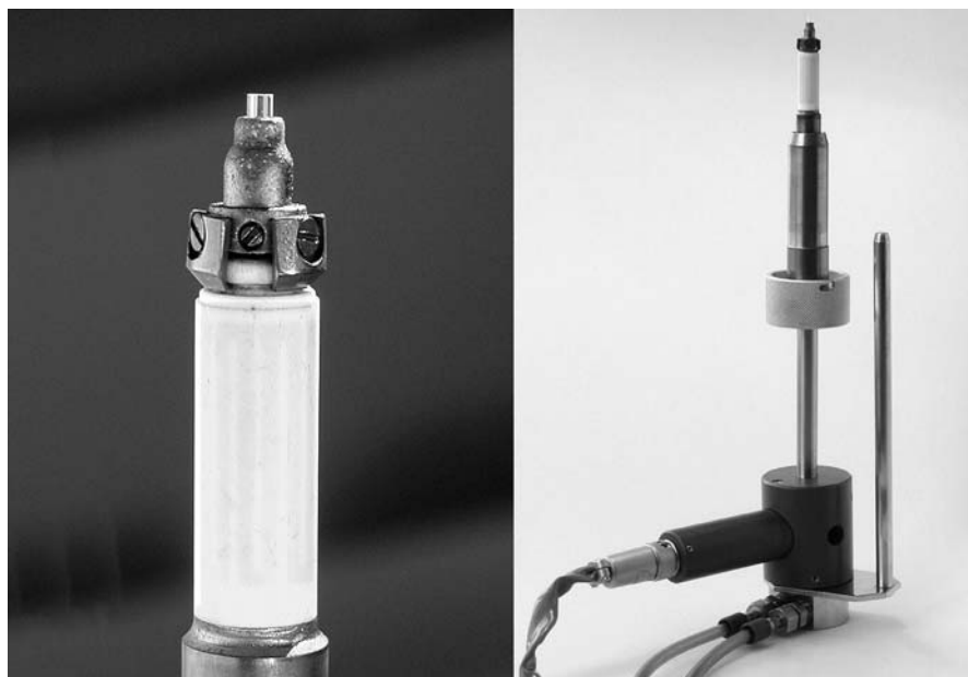
Fig. 5.12. DIP of a JEOL JMS-700 sector instrument for use with EI, chemical ionization (CI) and field ionization (FI). The copper probe tip holds the glass sample vial and is fitted to a temperature-controlled heater (left). The heater, a thermocouple, and circulation water cooling are provided inside. The (white) ceramics insulator protects the operator from the high voltage of the ion source.
