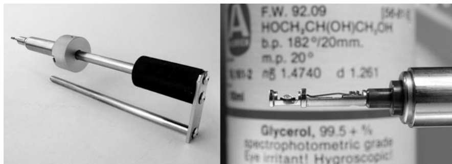
Fig. 9.3. FAB probe of a JEOL JMS-700 magnetic sector instrument (left). The probe tip with a drop of glycerol placed onto the exchangeable stainless steel FAB target (right).
