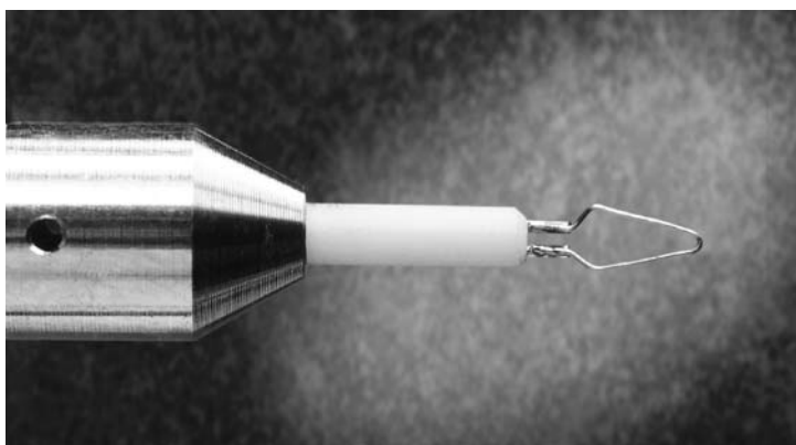
Fig. 5.16. Tip of a direct exposure probe of a GC- \alpha TOF mass spectrometer for EI, CI, FI). By courtesy of Waters Corporation, MS Technologies, Manchester, UK.
