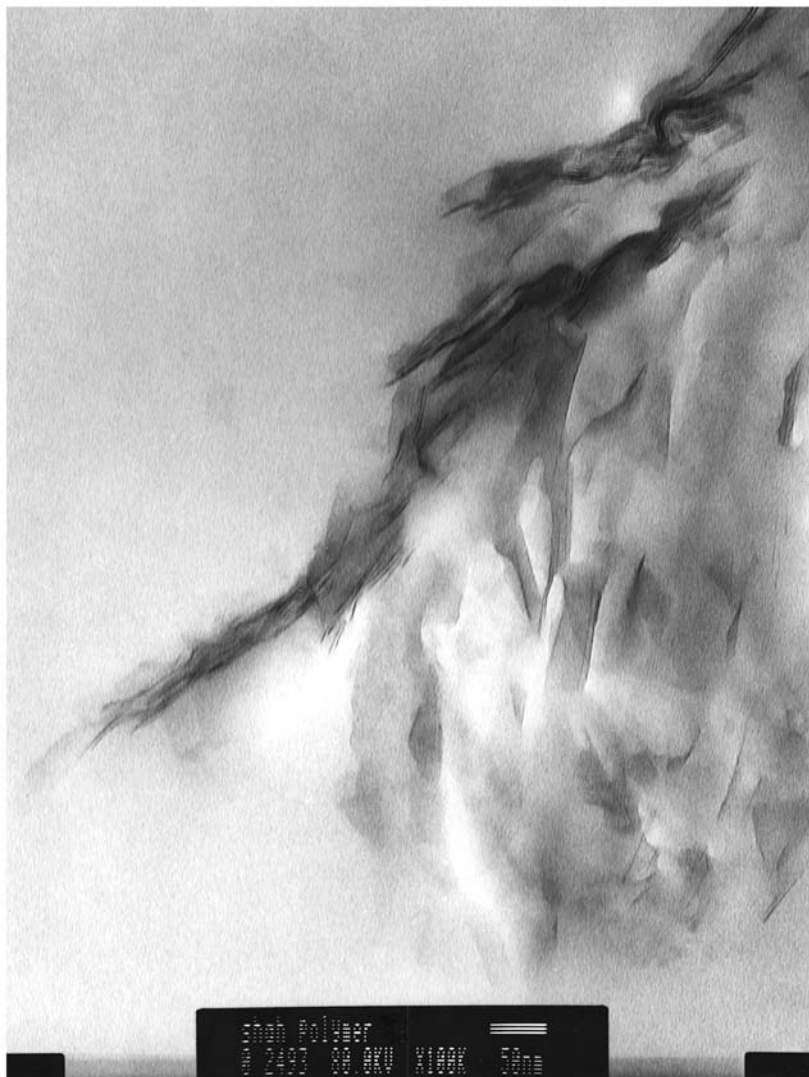
FIGURE 13.6 Transmission electron micrograph of vinyl ester/clay nanocomposite containing 0.5 wt% organically treated montmorillonite. The magnification is 100,000 \times . (From Ref. 37.)
